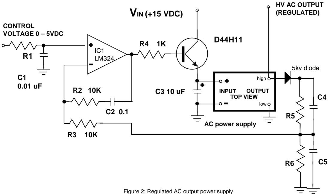
Figure 2: Regulated AC output power supply
