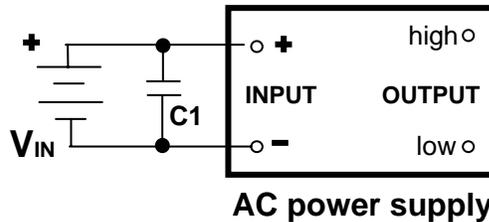
Figure 1: Basic AC hookup schematic (top view of AC shown)
