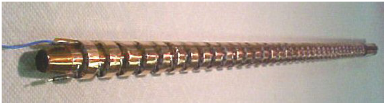
Figure 4: Tube and film arrangement showing elements of the 30 stage parallel multiplier.
