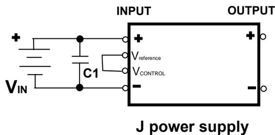
Figure 1: Basic J hookup schematic for maximum output
