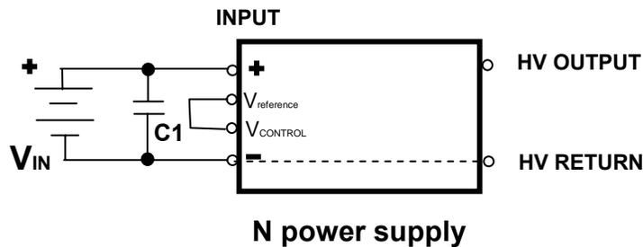
Figure 1: Basic N hookup schematic for maximum output
