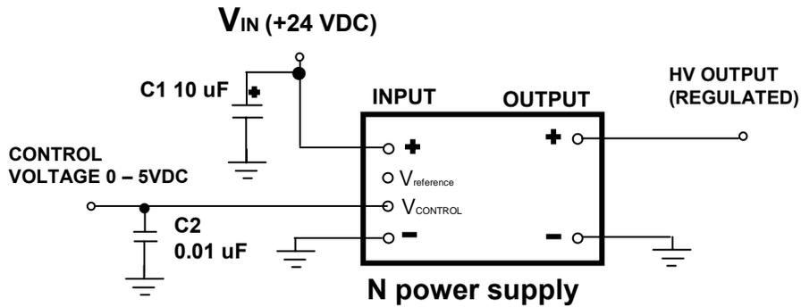
Figure 2: Voltage programming
