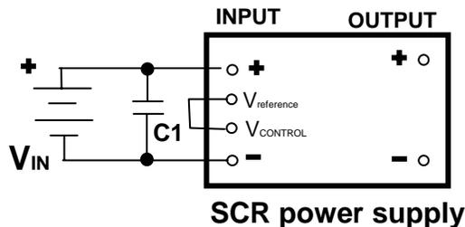
Figure 1: Basic SCR hookup schematic for maximum output
