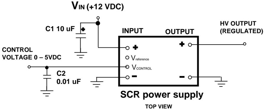
Figure 2: Voltage programming
