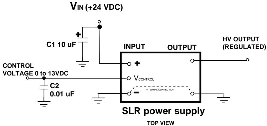
Figure 2: Voltage programming
