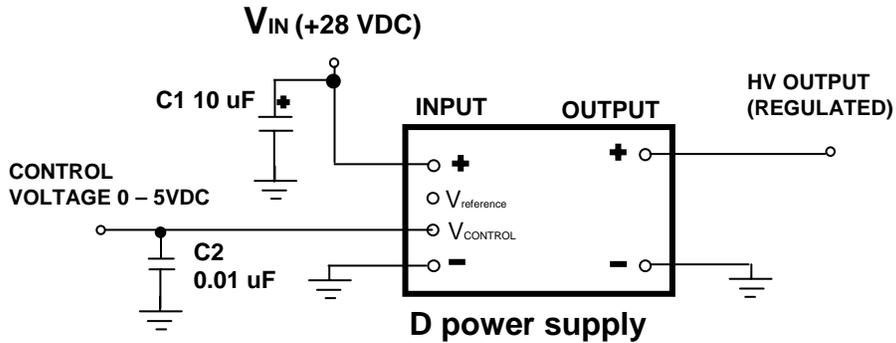
Figure 2: Voltage programming
